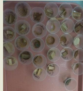
**Figure 3:** Final result depicting wood dust ready for dilution. Wood dust is pictured in plastic containers with respective solid wood samples
