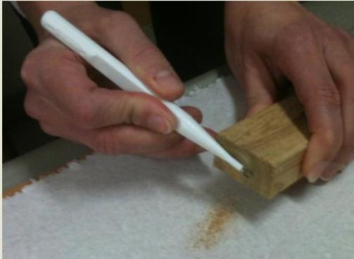
**Figure 1:** A disposable curette firmly drawn across the end grain of solid wood samples
